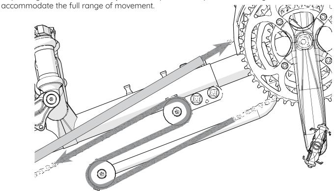
Adjust the chain to new routing and check length as outlined in the assembly manual. Fit the gear cable guide tube by pushing it over the gear cable housing (it has a split in it to allow for easy fitment) and secure it using cable ties. The gear cable out should be able to move freely as the boom is adjusted .
