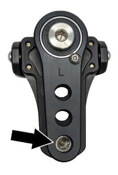
**4. Reattach the pedal**. Grease the threads and attach the pedal into the Pedal Swing as you normally would into a crank arm.
