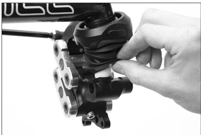
Slide off rubber gaiter at the bottom.
