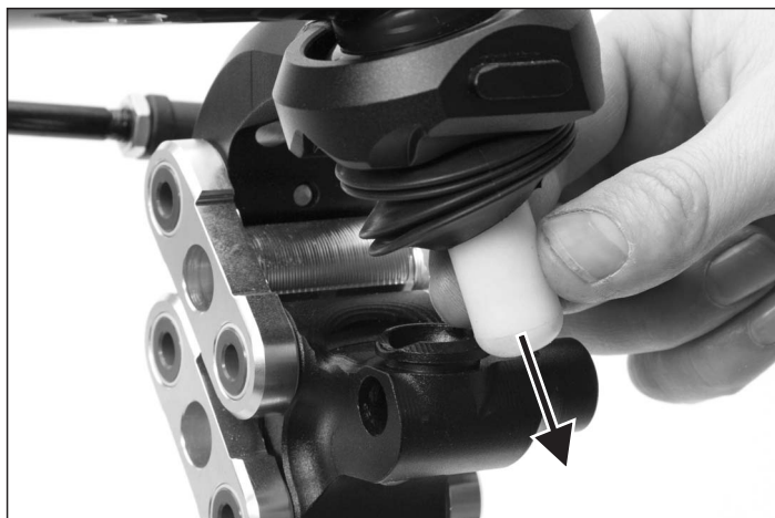
It should be easy now to pull out the elastomer fully.
