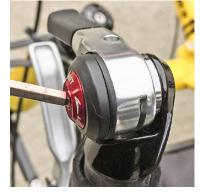
**3. Swing the shift lever aside.** You should now be able to see down inside the handlebar to the clamp that holds the shifter in place. Loosen the clamp bolt 1 (one!) turn. This should be enough to release the clamp. You don't want to overloosen the clamp as the parts may fall down inside the handlebar. Just barely loose is all you need. Note that some shifters (Microshift) are left hand threads-you'll have to turn clockwise to loosen them.
