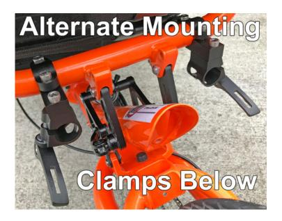
**3. Loosely Attach the Clamp.** Ensure the clamp isn't on a curving part of the tube. Tighten the 6mm bolts using a 5mm Allen wrench. Make sure the gap between the clamp faces is the same on both sides
