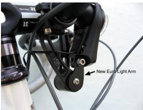
**Note:** Some lights will require a separate ground connector because the Accessory Mount is electrically isolated from the bike by the plastic Cateye clamps. Put the ground connector next to the light, on the bolt that holds the light itself.
