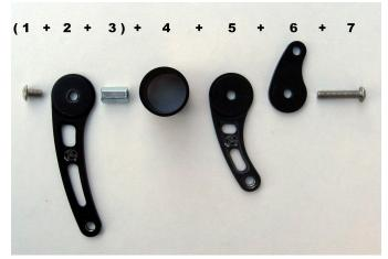
The Euro light mounting tab is part 6. Parts 1, 2, and 3 are fixed together, and then the other parts are attached. Parts 2 and 5 are curved and can be flipped around to work around obstacles.
