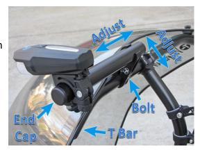
**4.** Adjust the position of the Light/Mirror mount tube. There are several options and just a few things to check. Basically, you can slide the Light/Mirror mount tube in and out and up and down to whatever position you'd like.
