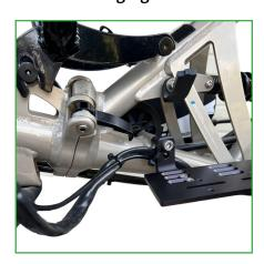
The Scorpion Battery Plate also includes additional threaded holes to install the Bosch Adapter Monorail as well as the STEPS Adapter Monorail!
