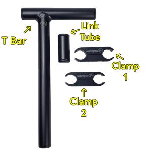
The clamps are 0.5" (12.7mm) tall and require only this much room to attach. It is best to attach the clamp to a straight section of tube. Attaching to a curving tube will not provide proper clamping and may dent the tube.
