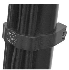
Be sure to check cable drape when turning the handlebars side to side, and if you have a folding stem, when folding the handlebars forward and back. When you've dialed things in, tighten the clamp bolts on the guides to to 20in-lb (2.5 N-m, medium hand tight). No need to overtighten.
